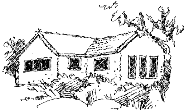
NOT THIS - Non-recessed windows do not cast any shadow, creating a "flat" facade.
